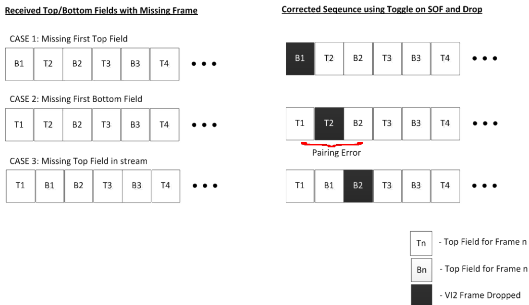
Figure 99: Error Correction for Interlaced Capture
